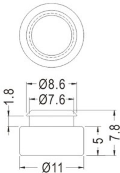
MOUNTING HOLE  $\text{Ø}7.0\sim\text{Ø}7.3$
